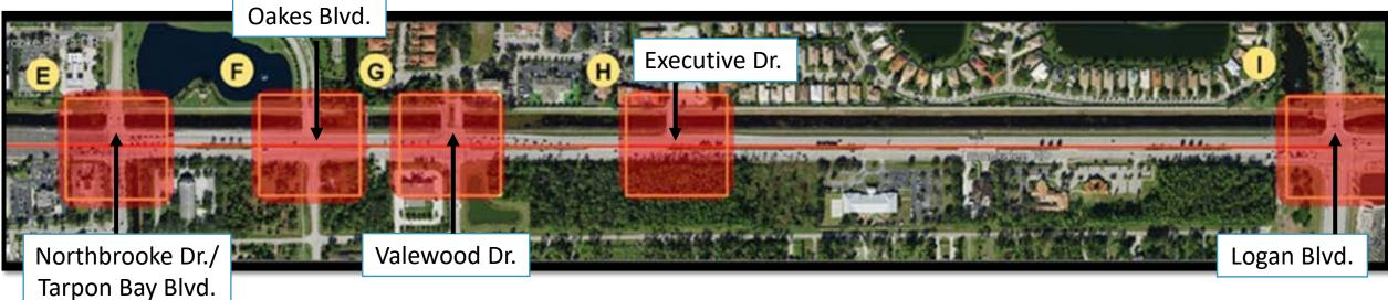
■ Improvements will be required along the entire corridor for it to operate efficiently. For example, the traffic flow at Intersection "A" (Livingston Rd.) influences the traffic flow at Intersections "B" through "I."
