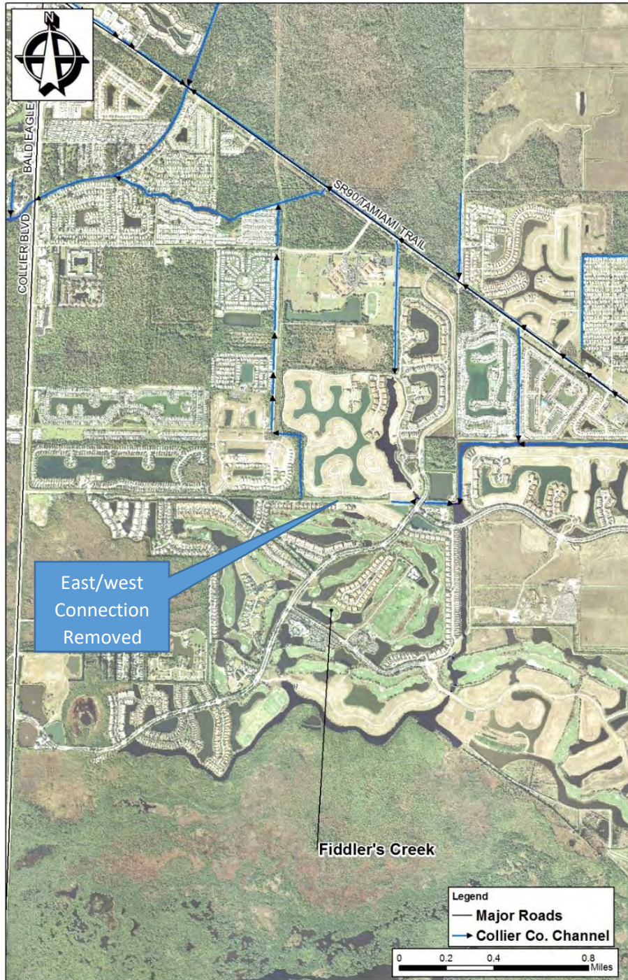
Figure 63. Collier County Stormwater Channel Network Near Fiddlers Creek
