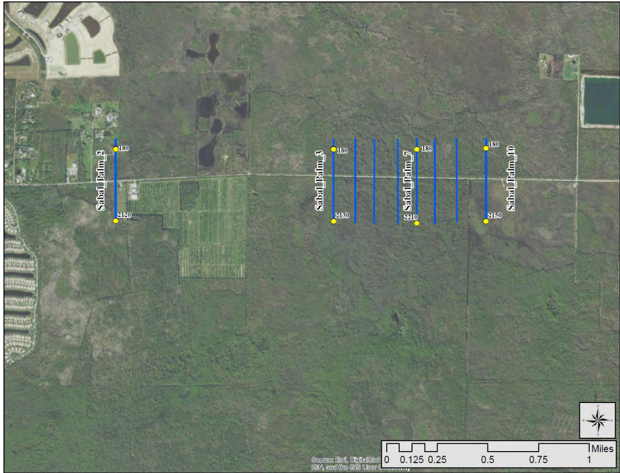
Figure 3.10 - Location of model calculation points along Sabal Palm Rd. at which 100-year maximum water levels are compared.
