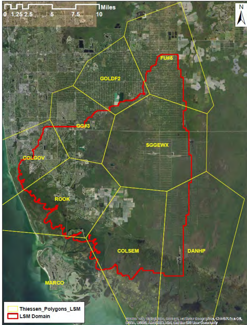
Figure 3.1 - Thiessen Polygons for design storm rainfall distribution over the modeled domain.
