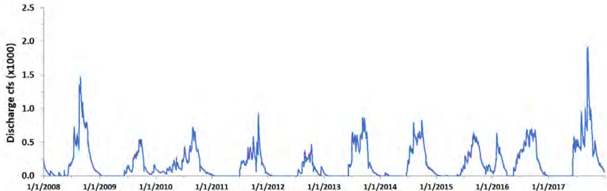
Figure 1.7 - Simulated discharges through the new GG-3 structure for the entire simulation period, 2008 to 2017.
