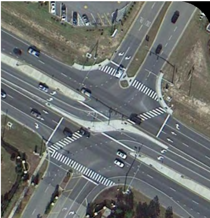
"Z" Pattern Crosswalk at an RCUT
