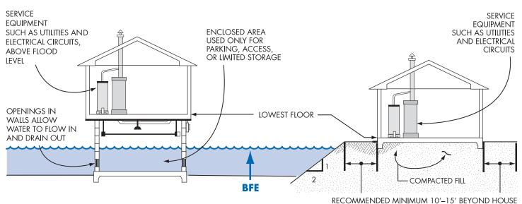
**CAUTION!** Enclosures (including crawlspaces) have some special requirements (see pages 40 and 41). Note: When the walking surface of the lowest floor is at the BFE, under-floor utilities are not allowed. Fill used to elevate buildings must be placed properly (see page 37).
