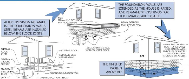
This is one way to elevate an existing building to comply with building code and floodplain regulations (also see FEMA P-312, *Homeowner's Guide to Retrofitting*). If an NFIP insured building is damaged by flood and the community determines it is substantially damaged, the owner may be eligible for an **Increased Cost of Compliance** payment (see page 56).
