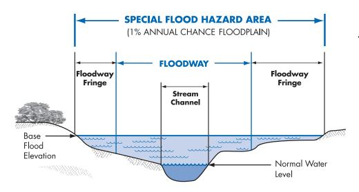
For floodplains with Base Flood Elevations (BFEs) determined by detailed flood studies, the Flood Profile in the Flood Insurance Study shows water surface elevations for different frequency floods (see page 12).
