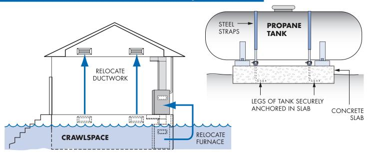
Move fuse boxes, water heaters, furnaces, and ductwork out of crawlspaces and basements. Anchor heating oil and propane gas tanks to prevent flotation and lateral movement. **Do not** store valuables or hazardous materials in a flood-prone crawlspace or basement. Use water-resistant materials when you repair.
