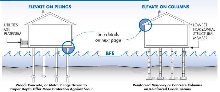
In Zone V, the design specifics will be determined by an architect or engineer based on the site, including how the building will be elevated and how deep the foundation elements will be in the ground. A Zone V Design Certificate or statement will be required (see page 32). For more information, see FEMA P-55, *Coastal Construction Manual*.
