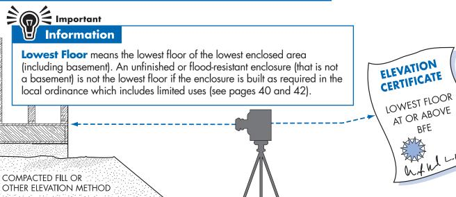
If you get a permit to build in a flood hazard area, a FEMA Elevation Certificate or a similar documentation will be required as soon as your lowest floor is set. An "as-built" survey and Elevation Certificate will be required when construction is completed. This form is important! It proves that you built correctly. It can be used to obtain the correct insurance rating.
