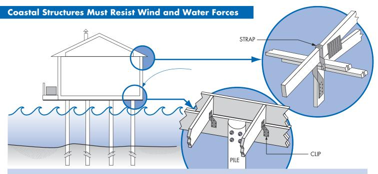
Coastal buildings may be exposed to hurricane winds, waves, and floodwaters. Structural building components must be connected together to transfer forces in a continuous load path from the roof to the foundation. The details above are some examples of how this is done. An architect or engineer must determine the types of connections required for the roof, building, and foundation.
