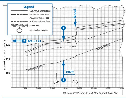
Flood Profiles from Flood Insurance Study reports can be used to determine the BFE at a specific site. Profiles also show estimated water surface elevations for floods other than the 1% annual chance flood (100-year).
