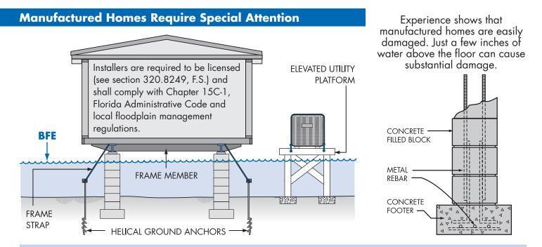
Homes must be anchored to resist flotation, collapse, and lateral movement by being tied down in accordance with your community's ordinance or the manufacturers' installation specifications for SFHAs. See guidance and some pre-engineered designs in FEMA P-85, Protecting Manufactured Homes from Floods and Other Hazards.
