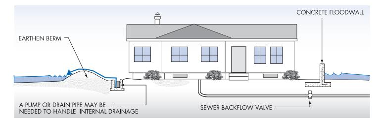
In areas where floodwaters aren't expected to be deep, sometimes individual buildings can be protected by earthen berms or concrete floodwalls. Permits are required for these protection measures and extra care must be taken if the site is in a floodway (see page 33). A small berm or floodwall does not remove elevation requirements and cannot be use to achieve compliance for a new or substantially improved building, or one that is repaired after substantial damage.
