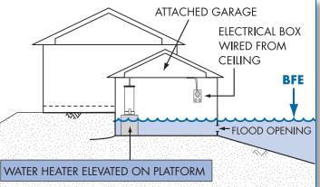
Appliances and equipment (including duct work) must be elevated to or above the BFE. Utilities (plumbing, electrical, gas lines, heating, ventilating and air conditioning) must be elevated or designed and installed to prevent intrusion of floodwaters into their components.
