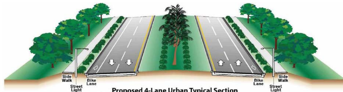
Proposed 4-Lane Urban Typical Section With Provisions for Median Expansion to 6 Lanes Randall Blvd Alternative
