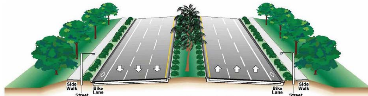
Proposed 6-Lane Urban Typical Section Randall Blvd Alternative
