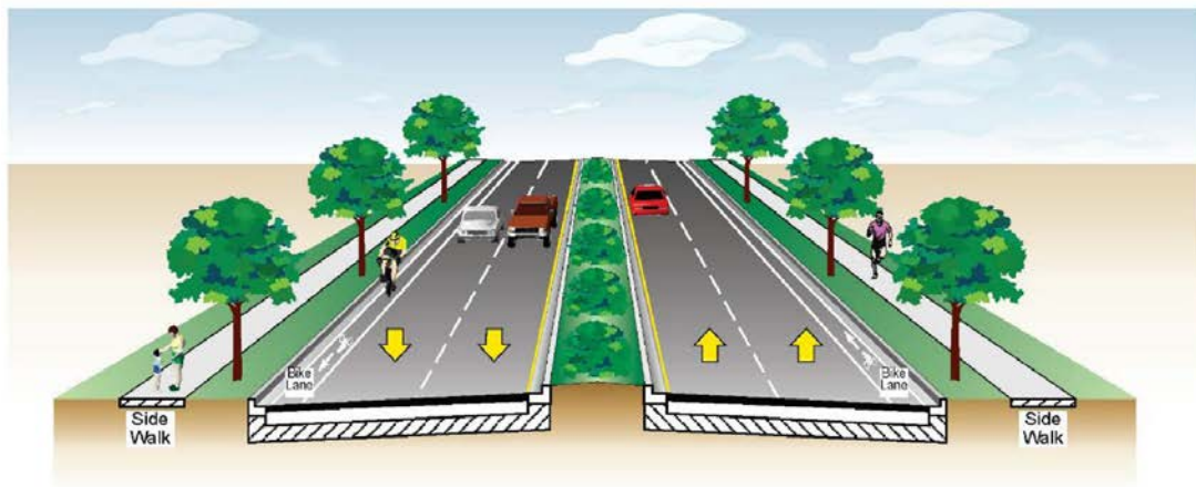
Proposed 4-Lane Urban Typical Section
