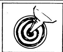
side edge applying an even bead around the entire edge and then work to the center.
