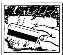
Clean application surface Apply adhesive to the back with wire brush. Surface of the marker as shown. must be clean, dry, and Start 1/8" in from the outfree of any loose debris. The presence of any foreign material (paint, oil, etc.) may affect adhesion.
