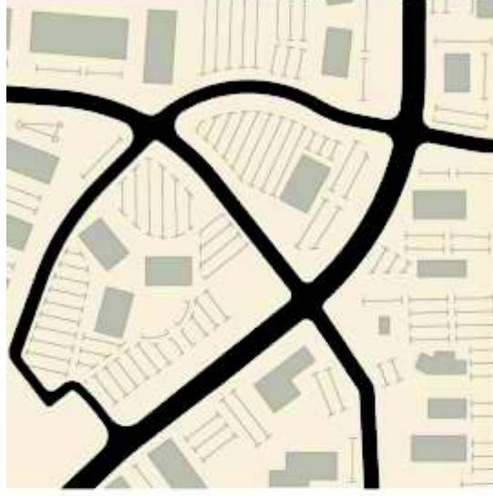
4-137. Lack of walkable block structure
