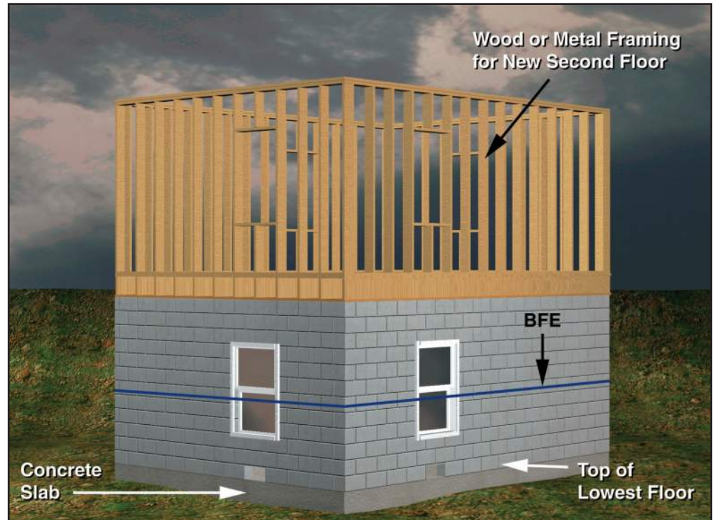
Figure 15 The new second-story floor and walls are built on top of the existing lower story.
