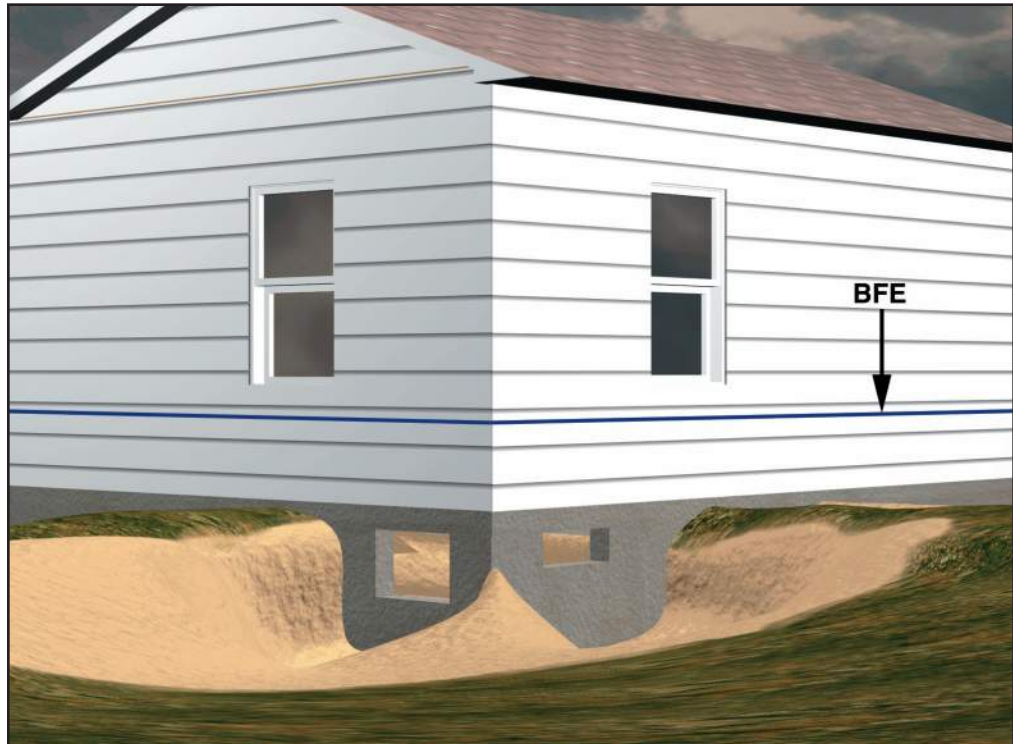
Figure 17 Trenches and tunnels under the slab provide access for the jacks and I-beams that will lift the house.
