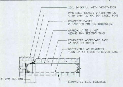
NOTE: THICKNESS OF GRAVEL BASE WILL VARY WITH TYPE OF SOIL SUBGRADE AND CLIMATE.
