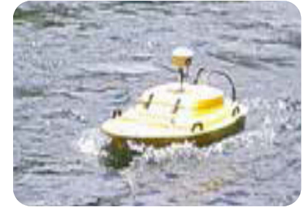
Photo 15- Z-Boat shown surveying a local canal.
