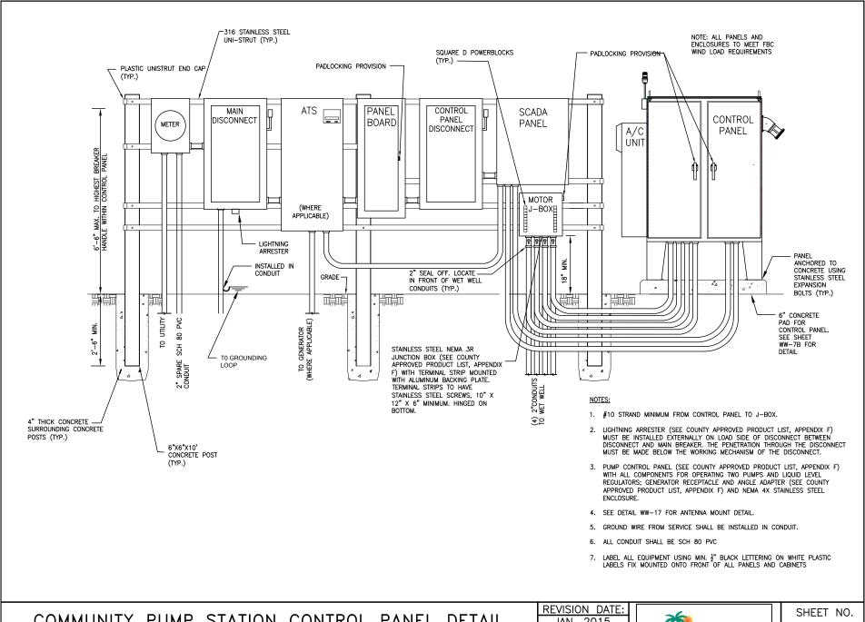
COMMUNITY PUMP STATION CONTROL PANEL DETAIL VFD STATION WITH GENERATOR
