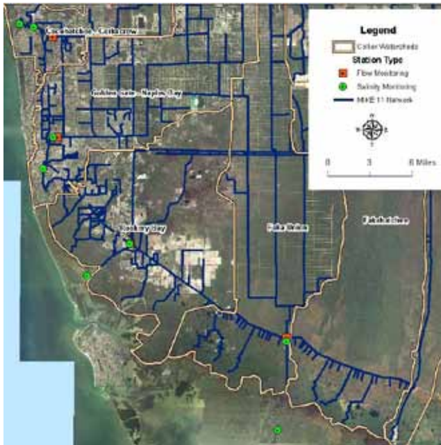
Figure 1-42. Flow and Salinity Monitoring Stations in Collier County
