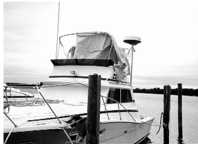
This boat was damaged by being slammed against the piling at its dock.
