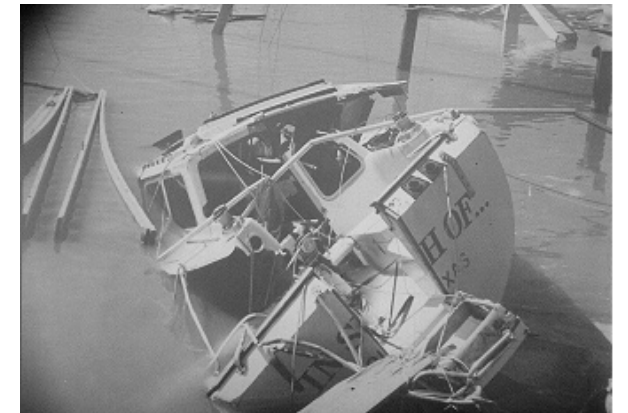
This boat broke apart at her dock with improper mooring lines.
