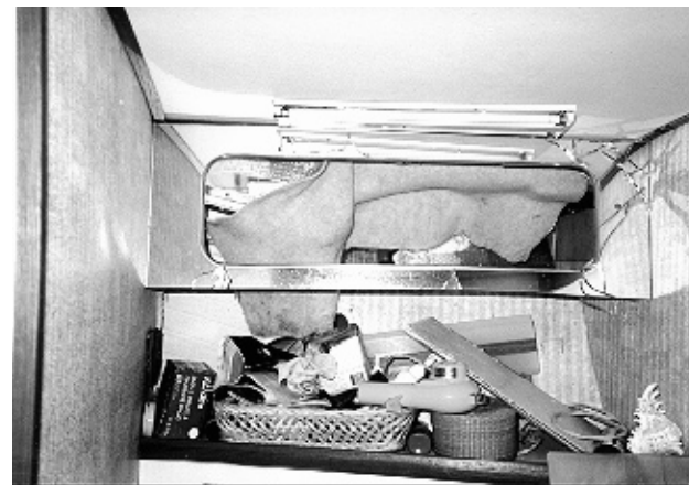
Note the broken mirror caused by the wrenching actions of the boat under buffeting waves and winds.
