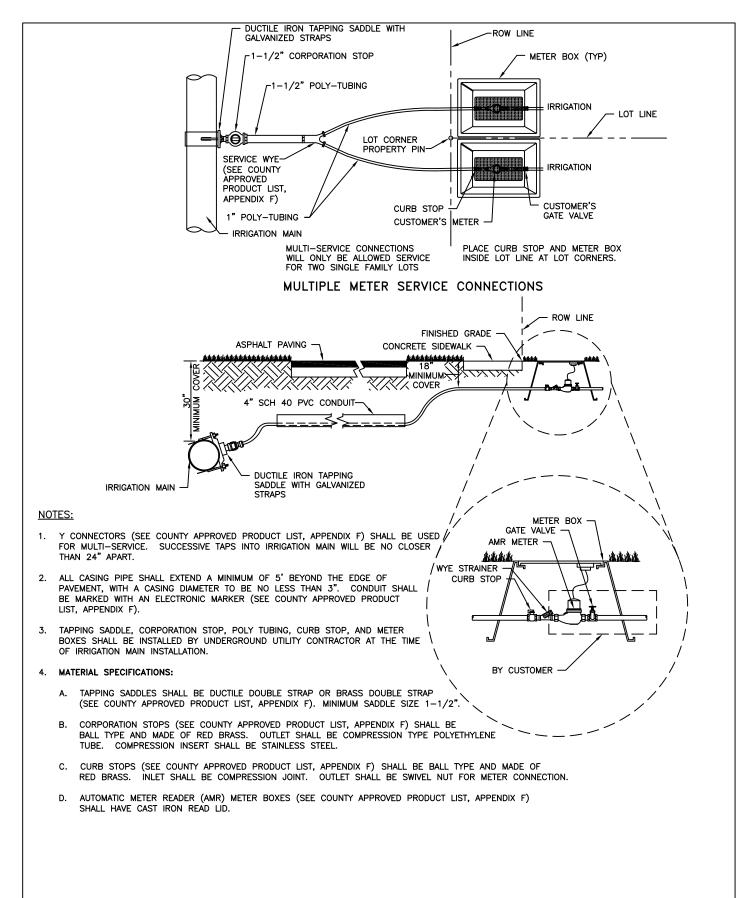
TYPICAL IRRIGATION SERVICE METER SETTING DETAIL FOR CONNECTION TO IRRIGATION MAIN
