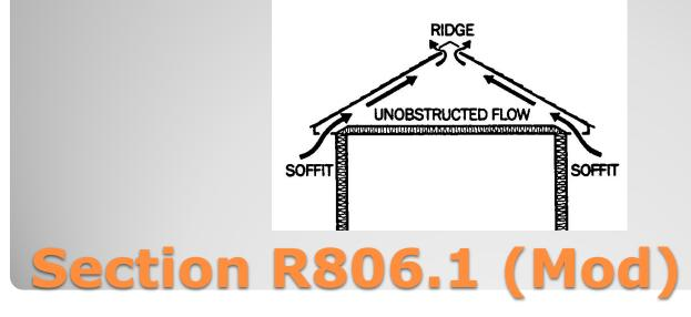
The net free cross-ventilation area may be reduced from 1/150 to 1/300 when a vapor barrier having a transmission rate not exceeding 1 perm is installed on the warm-in-winter side of the ceiling.
