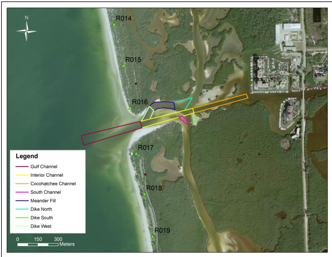
Figure 63. Components of the final alternative overlaying an aerial photograph of Wiggins Pass.
