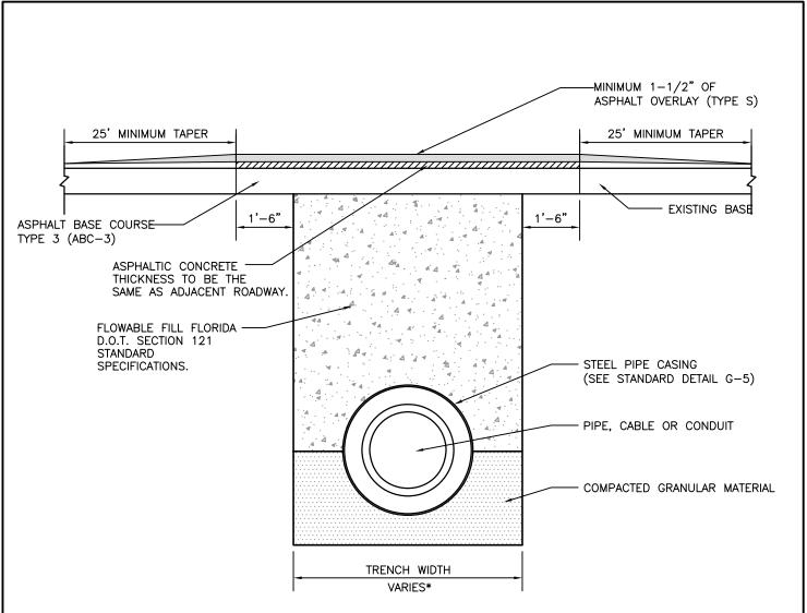
\*TRENCH WIDTH = PIPE OUTSIDE DIAMETER PLIS 2 FEET
