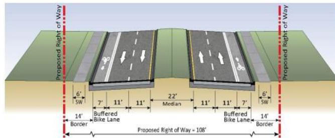
Figure 1.7 SR 29 Bypass Typical Section from CR 846 to Gopher Ridge Road
