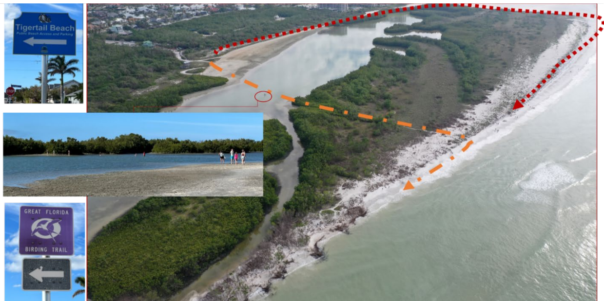
Public access pathways to gulf beach where the shoreline has retreated significantly and undermined dune
