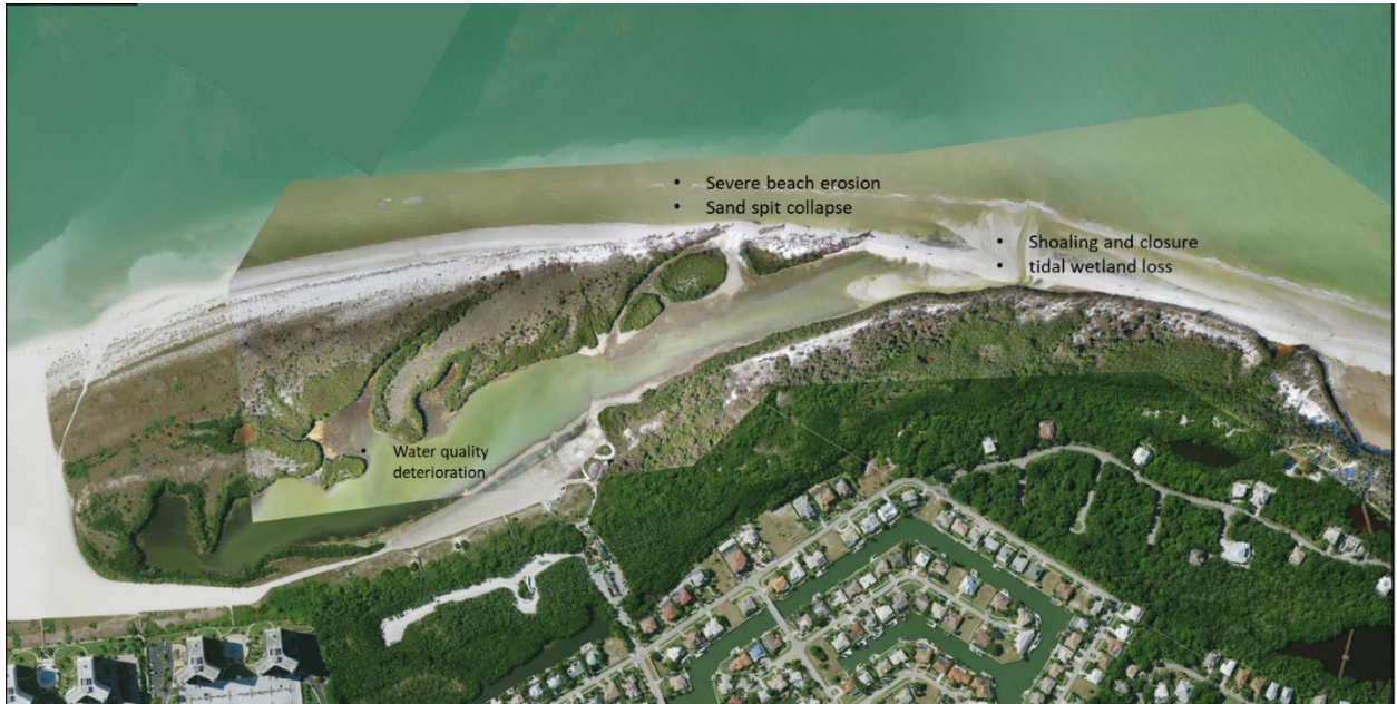
Existing conditions post Hurricane Ian at Tigertail Beach Park (October 2022)
