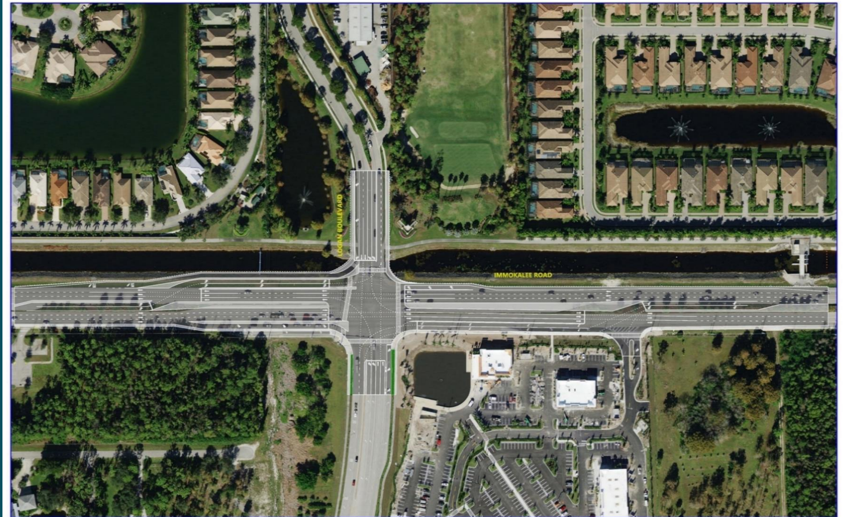
PARTIAL DISPLACED LEFT TURN IMMOKALEE ROAD AND LOGAN BOULEVARD INTERSECTION
