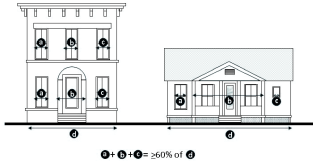
BGTCRA Redevelopment Area Figure 9 Building Façade Elevation Diagram (For illustrative purposes only)
